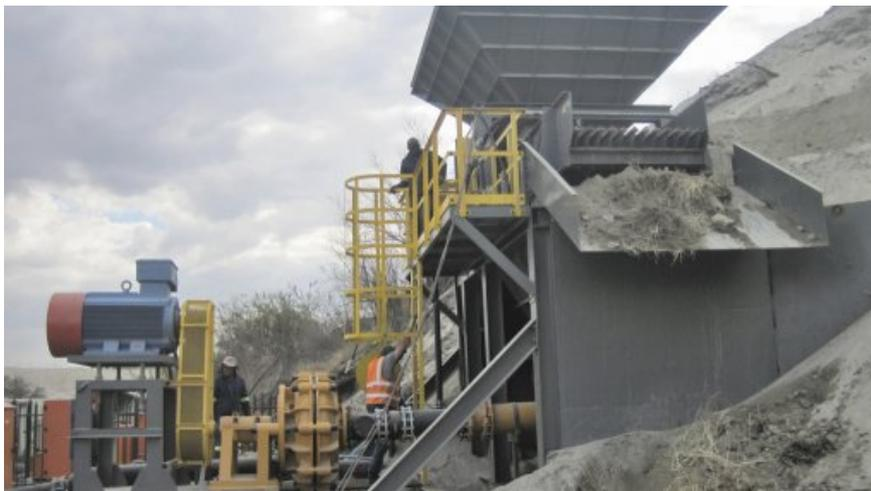
EASIER OPTION Jet-pump technology is being introduced for tailings reclamation owing to the difficulty of reclaiming coarse- and high-specific gravity tailings using conventional techniques
